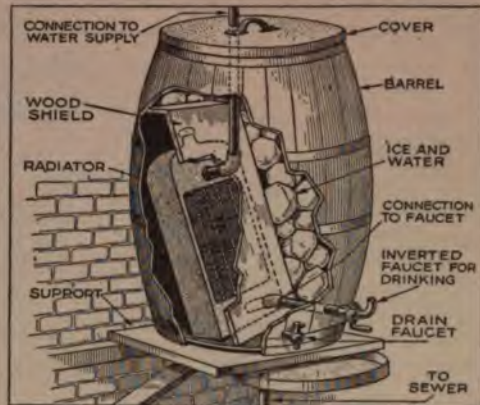
An Old Oil Barrel and a Discarded Radiator can be Combined to Furnish Cool Drinking Water
